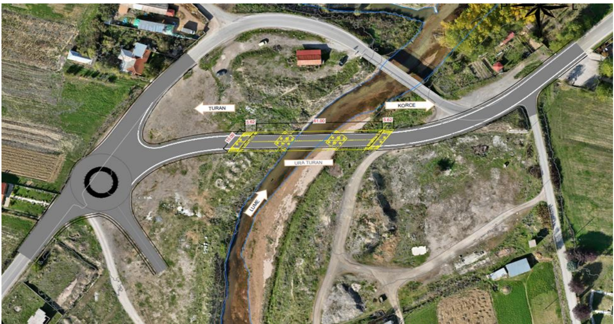
Figure 4: Aerial view of the existing bridge and the final design layout of the new bridge
